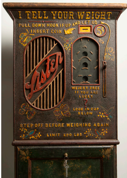
A rare 1903 scale played a phonographic recording of a person's weight for a nickel.
